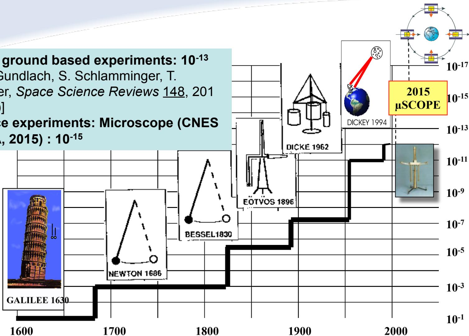
**objective: test of the Equivalence Principle between inertial mass and gravitational mass at  $10^{-15}$ , i.e. 2 to 3 orders of magnitude better than the best tests on ground**
