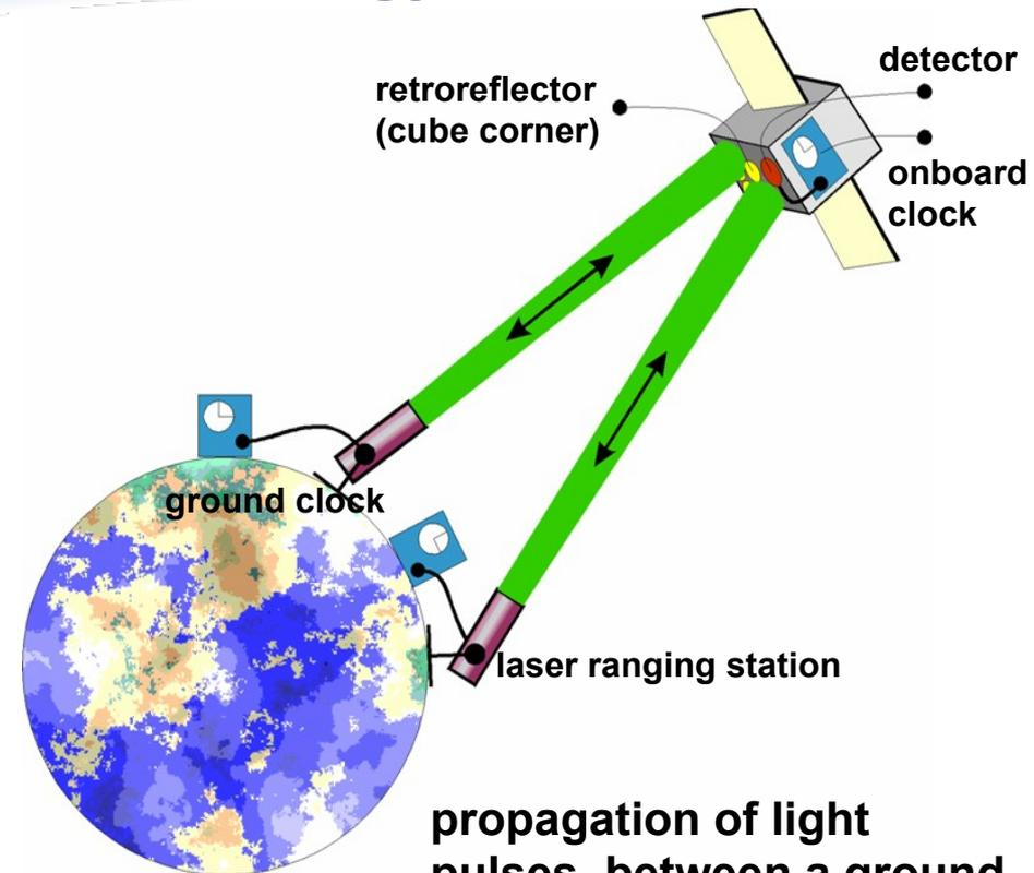
**propagation of light pulses between a ground based clock and a space clock**
