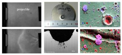
**Figure 3**: High velocity impact experiments on a metallic target with millimeter–sized basalt projectiles (left) using a two stages light gas gun (coll. Prof. A. Nakamura at the University of Kobe , Japan). In collaboration with CEMEF, target (center) and ejecta (left) are analyzed *post-mortem* for their microstructure and chemical composition. The ejecta (right), collected in an aluminium catcher were analysed for minor and trace elements using EDX-SEM and LA-ICPMS techniques.
