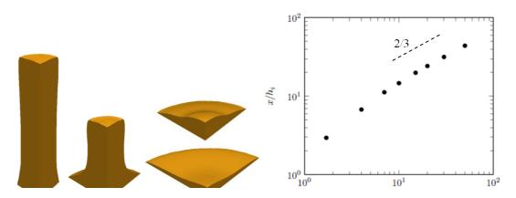
**Figure 5:** mu(I) computation of the shape of a granular column at t = 20%, 40%, 60% and 80% of total collapse and demonstration of the 2/3 scaling law of 2D relative spreading distance vs. initial aspect ratio.
