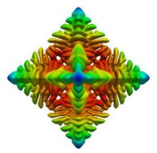
Figure 4. Phase field simulation of dendritic growth in an undercooled melt revealing the overal morphology of the primary solid phase formed from the melt [3].
