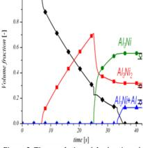
Figure 2. Time evolution of the fraction of phases (full symbols) predicted and (open symbols at 42 s) measured for the same sample as in Figure 1 [1].
