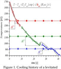
Figure 1. Cooling history of a levitated Ni-75at.%Al 6 mm diameter droplet (colored curve) measured and (grey) calculated (DLR, Köln, DE) [1].
