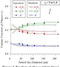
Figure 3. Fraction of phases (plain lines) predicted and (dashed lines) measured using neutron diffraction (Aix-Marseille University) in atomized particles [2].
