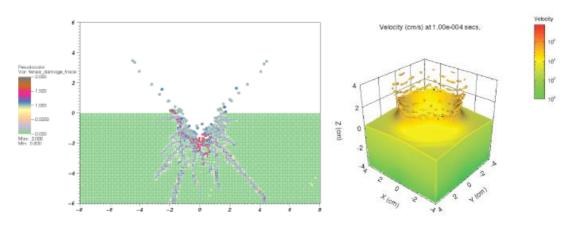
**Figure 2:** left: simulation results from a calculation by the Spheral ++ SPH code (see Theme 11.5) of a 0.635 cm basalt impactor impacting at 5 km/s onto a basalt half-space. The colored contours show the trace of the damage tensor, where 2 (brown/black is fully damaged. Right: Same from a calculation using the adaptive grid-code CTH. Colors show velocity contours, allowing the velocity of ejecta particles to be tracked and quantified (from Stickle et al. 2016).
