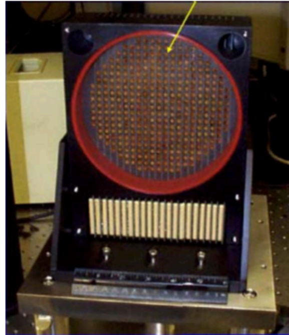
349 actuators on 7 mm spacing
